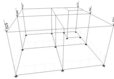
**Figure 6.** Modeling of gravity loads.
