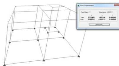
**Figure 7.** Deformed shape of house (unit mm).
