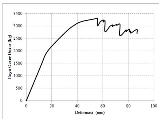
**Figure 9.** Capacity curves (note in Indonesian).
