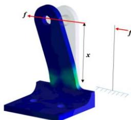
**Figure 3.** Plastic moment reached in the end of the energy plate
