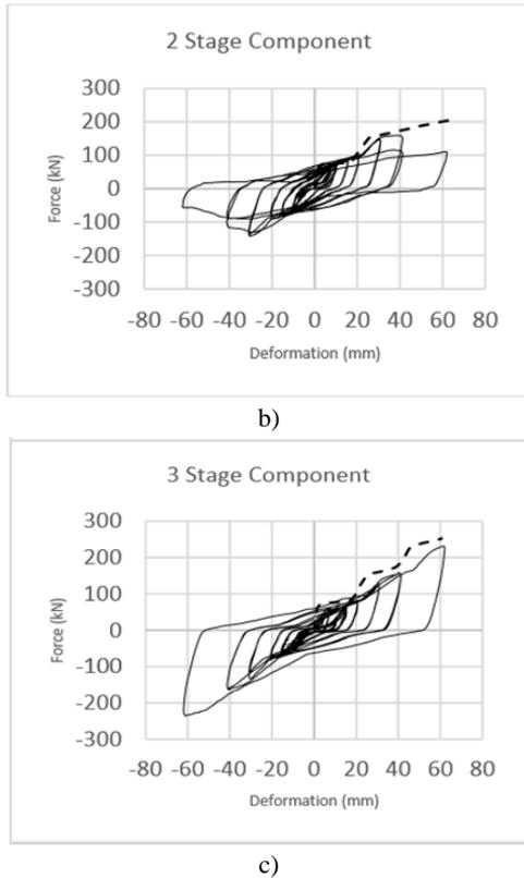
**Figure 7.** a) 1SC, b) 2SC, c) 3SC, comparison experiment result and FEM result
