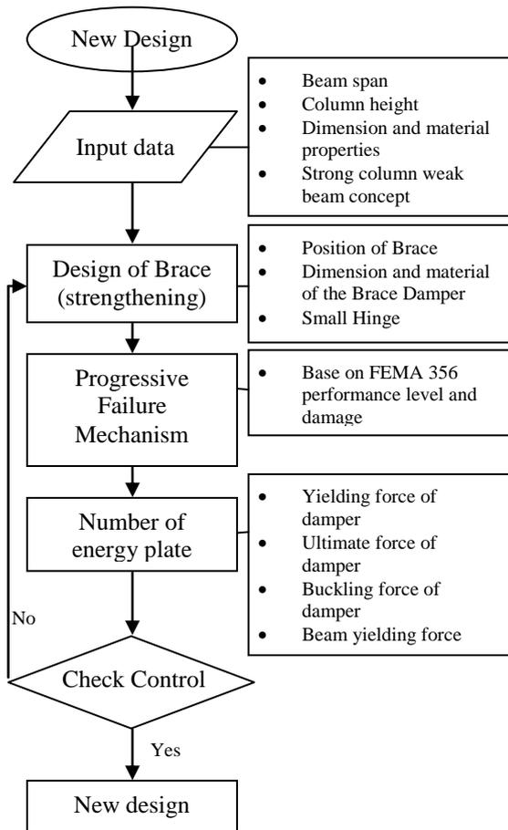
**Figure 1.** Design Procedure
