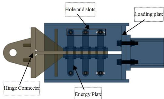
**Figure 5.** Detail of Brace Damper Configuration
