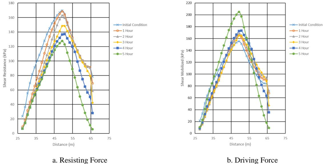
**Figure 7.** Resisting force and driving force at the sliding surface
