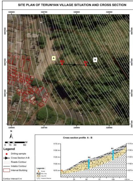
a. Cross section A-B and Drilling sample
