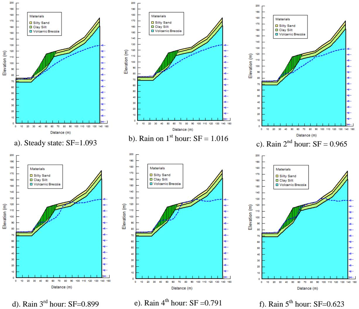
**Figure 5.** Safety factor and ground water level
