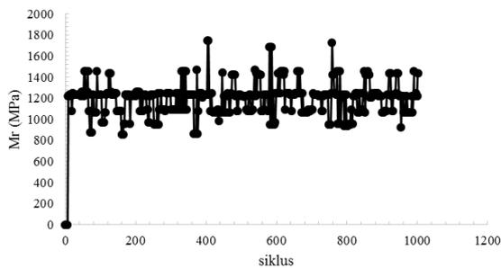
**Figure 7.** Addition of 20% Merapi volcanic ash and 3% lime stage conditioning Resilient Modulus.
