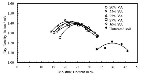
**Figure 5.** Graph of standard proctor result on original soil and soil mixed with volcanic ash of Merapi volcano and 3% of lime
