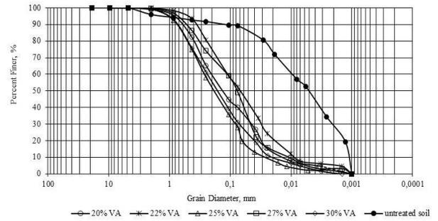
**Figure 4.** Graph of addition of Merapi volcanic ash and 5% of lime against grain size distribution
