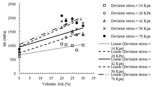
**Figure 9.** Influence the addition of volcanic ash of Merapi and 5% of lime to Resilient Modulus at  $\sigma_3 = 42$  kPa.
