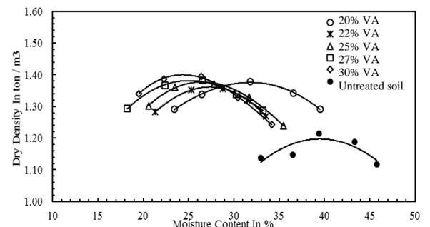
**Figure 6.** Graph of standard proctor result on original soil and soil mixed with the volcanic ash of Merapi volcano and 5% of lime.
