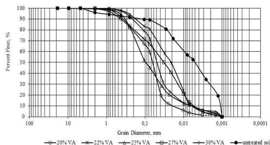
**Figure 3.** Graph of addition of Merapi volcanic ash and 3% of lime against grain size distribution
