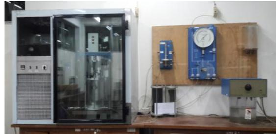
**Figure 1** Triaxial Test Apparatus
