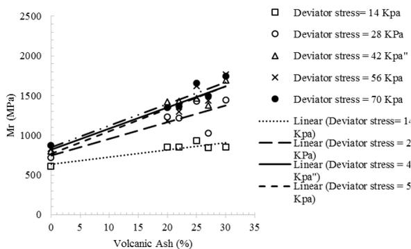
**Figure 8.** Influence the addition of volcanic ash of Merapi and 3% of lime to Resilient Modulus at  $\sigma_3 = 42$  kPa.
