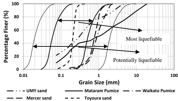
Figure 5. Particle size distribution of soil sample
