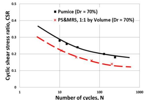
**Figure 3.** Comparison of CSR values from mixed Waikato pumice with Mercer sand, and Toyoura sand at the same relative density (Liu et al., 2015)
