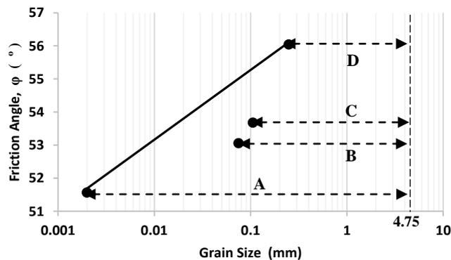
Figure 9. Shear strength behavior of Mataram pumice
