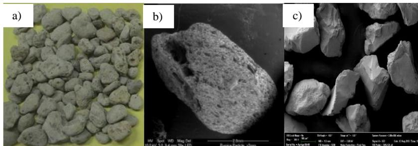
**Figure 4.** a) Mataram Pumice, retained #10 sieve (grain size 4.75 – 9.52 mm),
