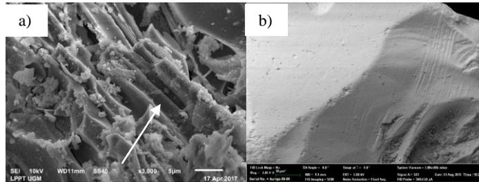
**Figure 6.** SEM micrograph showing: a) the internal voids in Mataram pumice, b) Toyoura sand (Alshibli K., 2013)
