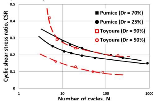
**Figure 2.** Comparison of CSR values from Waikato Pumice and Toyoura sand with different densities (Liu, et al., 2015)
