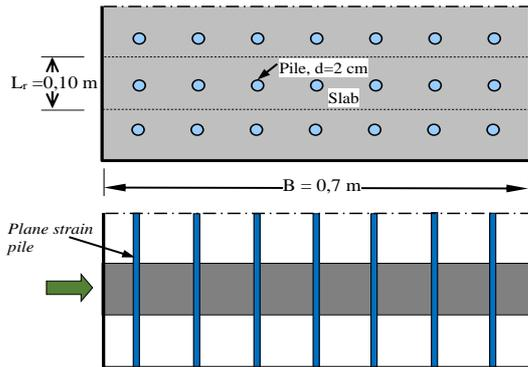
Figure 1. Plane strain model for slabs with piles
