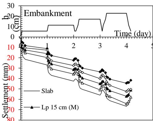
**Figure 9.** Effect of load increment to settlement at the center for uniform load
