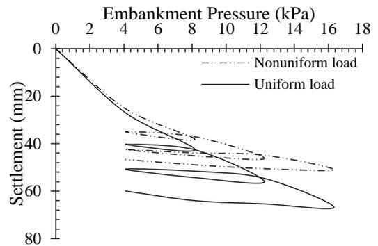
**Figure 12.** Relation between pressure and settlement of slab
