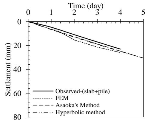
**Figure 18.** Comparison between calculated and observed settlement of slab with 35cm piles center loading
