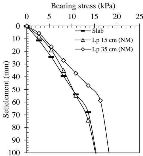
**Figure 5.** Bearing stress-settlement at the center curves for slab with non-monolithic piles
