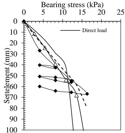
**Figure 6.** Typical settlement data at the center under different load rate
