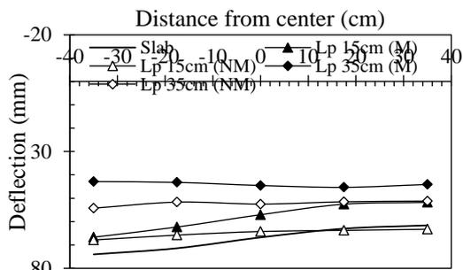
**Figure 11.** Deflection along slab for the uniform load of 16.33 kPa
