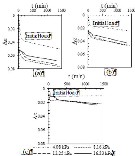
**Figure 16.** Compression after unloading on slabs: (a) without piles; (b) 15-cm piles; (c) 35-cm piles
