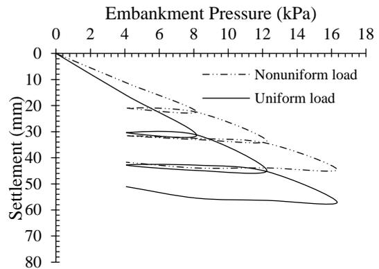
**Figure 14.** Relation between pressure and settlement of slab with 35-cm piles
