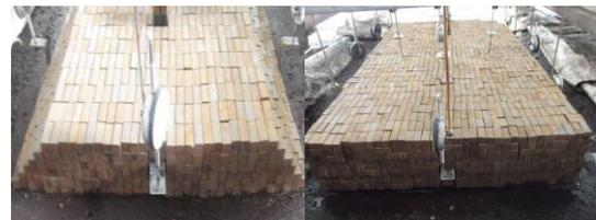
Figure 3. Photographs of embankment model test: (a) Non-uniform load; (b) Uniform load
