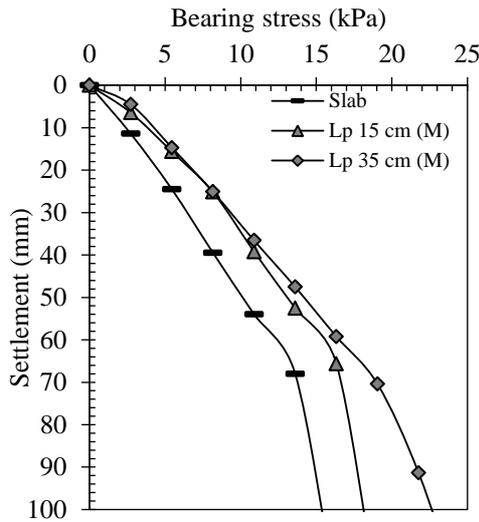
**Figure 4.** Bearing stress-settlement at the center curves for slab with monolithic piles
