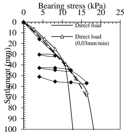
**Figure 7.** Typical settlement data at slabs with 15-cm piles under different load conditions
