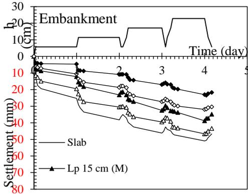
**Figure 8.** Effect of load increment to settlement at the center for non-uniform load
