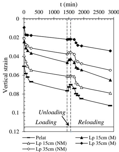
**Figure 15.** Relation between time and strain under loading-unloading
