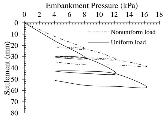
**Figure 13.** Relation between pressure and settlement of slab with 15-cm piles
