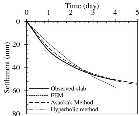
**Figure 17.** Comparison between calculated and observed settlement of slab for center loading
