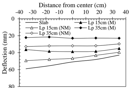
**Figure 10.** Deflection along slab for non-uniform load of 16.33 kPa
